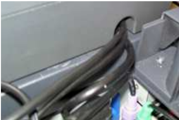
Figure 8, Printer Cables Routing
